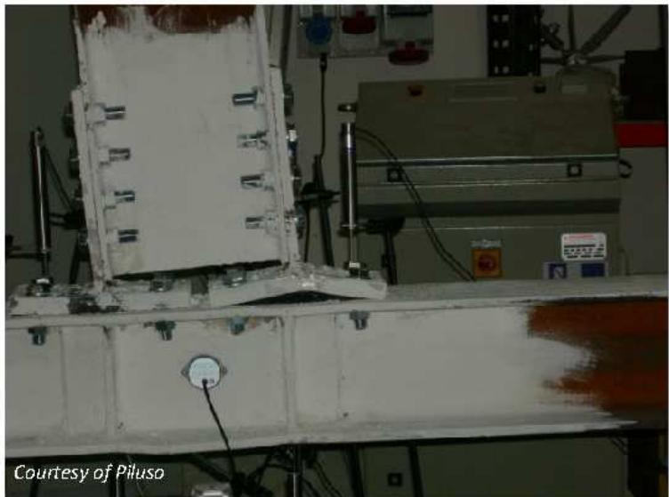
When dissipative zones are located **in the connections**, the connected members shall have sufficient overstrength to allow the development of cyclic yielding in the connections
